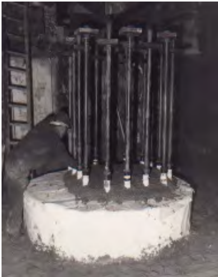
Figure 2 – Sensing pillars of the load cell
