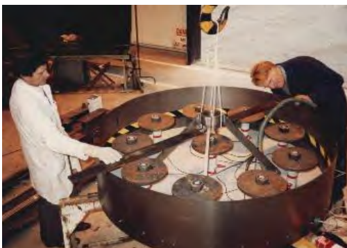
Figure 4 – Base load cell with sensing elements and pressure pad
