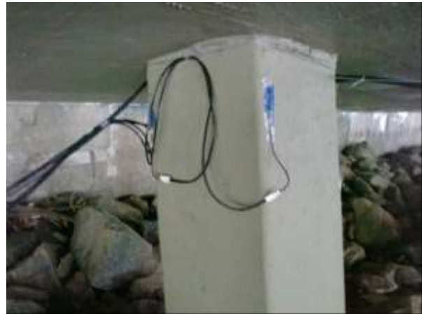
Figure 6 – Strain gages in piles P2 and P3
