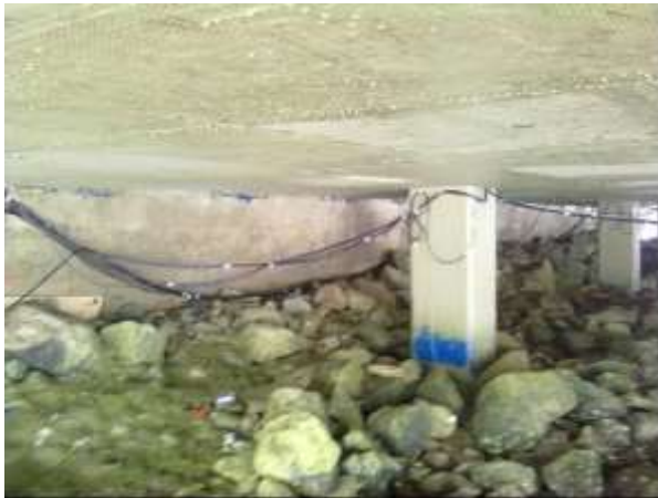
Figure 6 – Strain gages in piles P2 and P3
